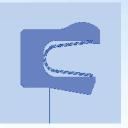
URV Rod Seal | Shaft Seal For fluids.
