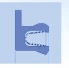
URF – Shaft and Rod Seal With clamping flange for sealing rotary and swiveling applications.
