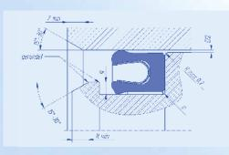
Installation into semi-closed groove (Snap-in assembly)
