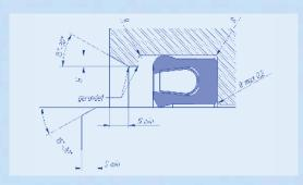
Installation into semi-closed groove (Snap-in assembly)
