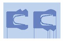
**Piston and Rod Seal** For critical fluids (paint, lacquers, gasoline, etc.).
